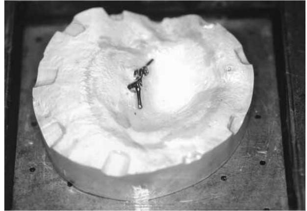
Fig. 1. Polyurethane sheet vacuum formed over perforated cast.
