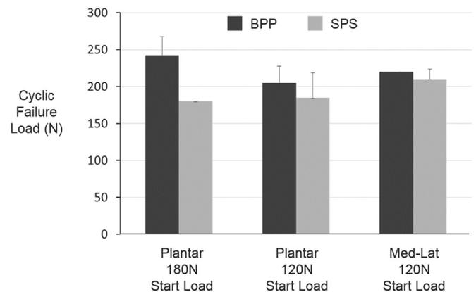
Fig. 6. Cyclic failure load for the different combinations of load direction and starting load magnitude. Note that the biplane plating construct (BPP; black bar) failure load was significantly greater than the single locking plate construct (SPS; gray bar) for cyclic plantar loading starting at 180 N.
