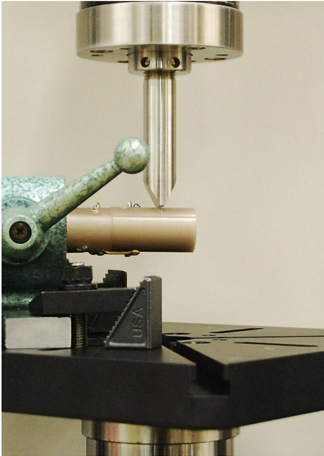
Fig. 3. Test setup for mechanical testing of static and cyclic cantilever bending.
