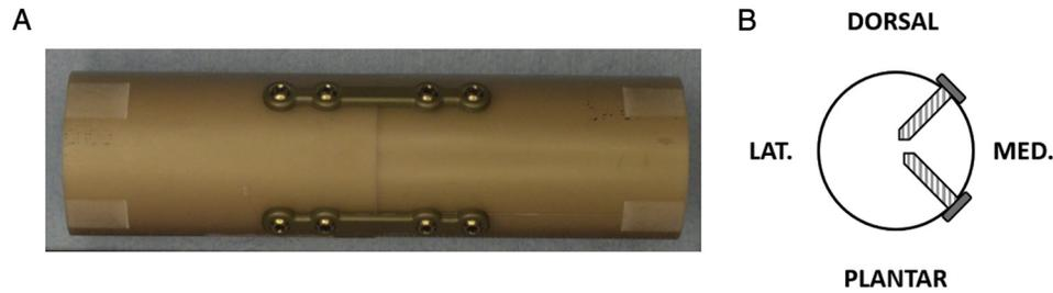
**Fig. 1.** Image of a test specimen (A) and schematic of the cross-section (B) of the biplane plating construct with dorsomedial and medial–plantar plates fixated unicortically with  $2.5 \times 14$ -mm locking screws. LAT, lateral; MED, medial.
