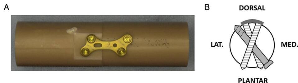
**Fig. 2.** Image of a test specimen (A) and schematic of the cross-section (B) of the single locking plate construct with anatomic Lapidus locking plate placed dorsally with four 3.5-mm locking screws engaged bicortically and a single 4.0-mm interfragmentary screw engaged bicortically. LAT, lateral; MED, medial.
