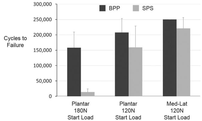
Fig. 5. Number of cycles to failure for the different combinations of load direction and starting load magnitude. Note that biplane plating construct (BPP; black bar) cycles to failure was significantly greater than the single locking plate construct (SPS; gray bar) for cyclic plantar loading starting at 180 N.
