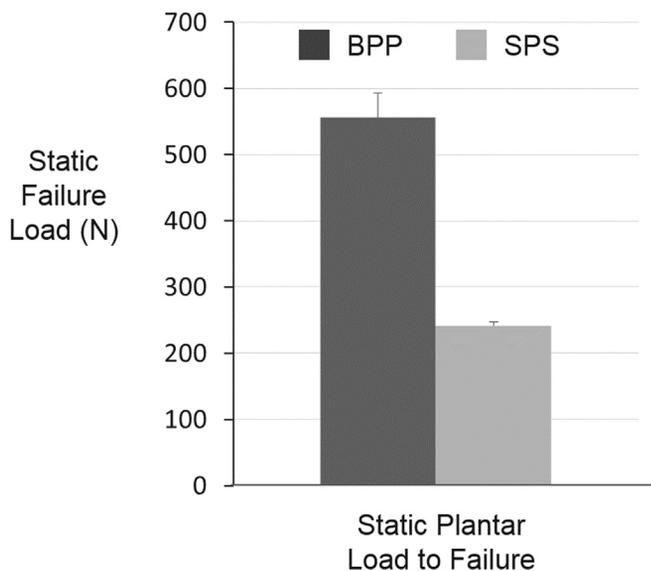
Fig. 4. Static ultimate failure load under plantar bending for the biplane plating (BPP) construct (black bar) and single locking plate (SPS) construct (gray bar). Note that the BPP failure load was significantly greater than the SPS.
